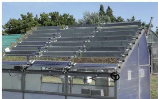
图 1 温室南坡面覆盖可沿纵向轴线旋转的晶体硅光伏板 Fig. 1 Covering crystal silicon photovoltaic panels which can rotate along the longitudinal axis on greenhouse south slope
