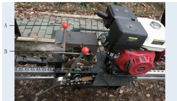
注:A.前进/后退机械推杆;B.运行/刹车机械推杆 Note:A.Forward/backward mechanical putter;B.Running/brake mechanical putter
